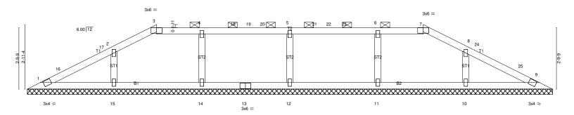
Plate Offsets (X,Y)-- [3:0-3-0,Edge], [7:0-3-0,Edge] LOADING (psf) CSI. SPACING-DEFL. **PLATES GRIP** 2-0-0 L/d in (loc) I/defI TCLL (roof) 47.0 Plate Grip DOL 1.15 TC 0.46 Vert(LL) 999 MT20 197/14 n/a n/a Snow (Pf/Pg) 46.2/60.0 Lumber DOL 1.15 BC 0.13 Vert(CT) n/a 999 n/a TCDL 7.0 WB Rep Stress Incr YES 0.18 Horz(CT) 0.01 9 n/a n/a **BCLL** 0.0 Code IRC2015/TPI2014 Matrix-S Weight: 65 lb **BCDL** 10.0
