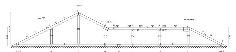
Plate Offsets (X,Y)-- [7:0-6-10,Edge] LOADING (psf) SPACING-CSI. DEFL. **PLATES GRIP** 2-0-0 L/d in (loc) I/defI TCLL (roof) 47.0 Plate Grip DOL 1.15 TC 0.96 Vert(LL) 999 MT20 197/14 n/a n/a Snow (Pf/Pg) 46.2/60.0 Lumber DOL 1.15 BC 0.34 Vert(CT) n/a 999 MT18HS 197/14 n/a TCDL 7.0 Rep Stress Incr WB YES 0.23 Horz(CT) 0.00 8 n/a n/a **BCLL** 0.0
