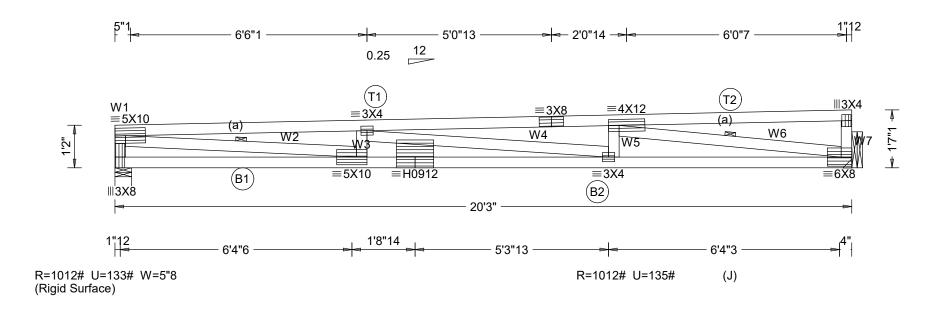
LEFT JIG = 20'3"12 RIGHT JIG = 20'3"6 SEQ = 130030 SCALE =0.3880 QTY= 15 TOTAL= 15 REV. 21.01.03A.0805.14 PLT. TYP.-WAVE DESIGN CRIT=IBC2018/TPI-2014 FT/RT=20%(0%)/ 0(0) 30.0psf REF TC LL 10.0psf TC DL DATE THIS DRAWING SHOULD BE APPROVED BY A REGISTERED 10.0psf BC DL DRWG 10-21-2022 PROFESSIONAL ENGINEER BEFORE USE. SEE PAGE A100 0.0psf BC LL FOR GENERAL NOTES, IMPORTANT SPECIFICATIONS AND 50.0psf TOT.LD. O/A LEN. 200300 WARNINGS. 1.15 JOB #: 13774 DUR.FAC SPACING 24.0" MONO **TYPE**
