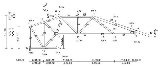
2-00-00 CSI DEFI (loc) I/defl I/d **PLATES** GRIP Loading (psf) Spacing in 40.0 Plate Grip DOL 1.15 TC 0.71 Vert(LL) -0.19 11-13 >999 240 MT20 197/144 (Roof Snow = 40.0) Lumber DOL 1.15 вс 0.97 Vert(CT) -0.38 11-13 >795 180 **TCDL** 10.0 Rep Stress Incr YES WB 0.37 Horz(CT) 0.16 n/a 9 n/a Code IRC2015/TPI2014 **BCLL** 0.0 Matrix-MS
